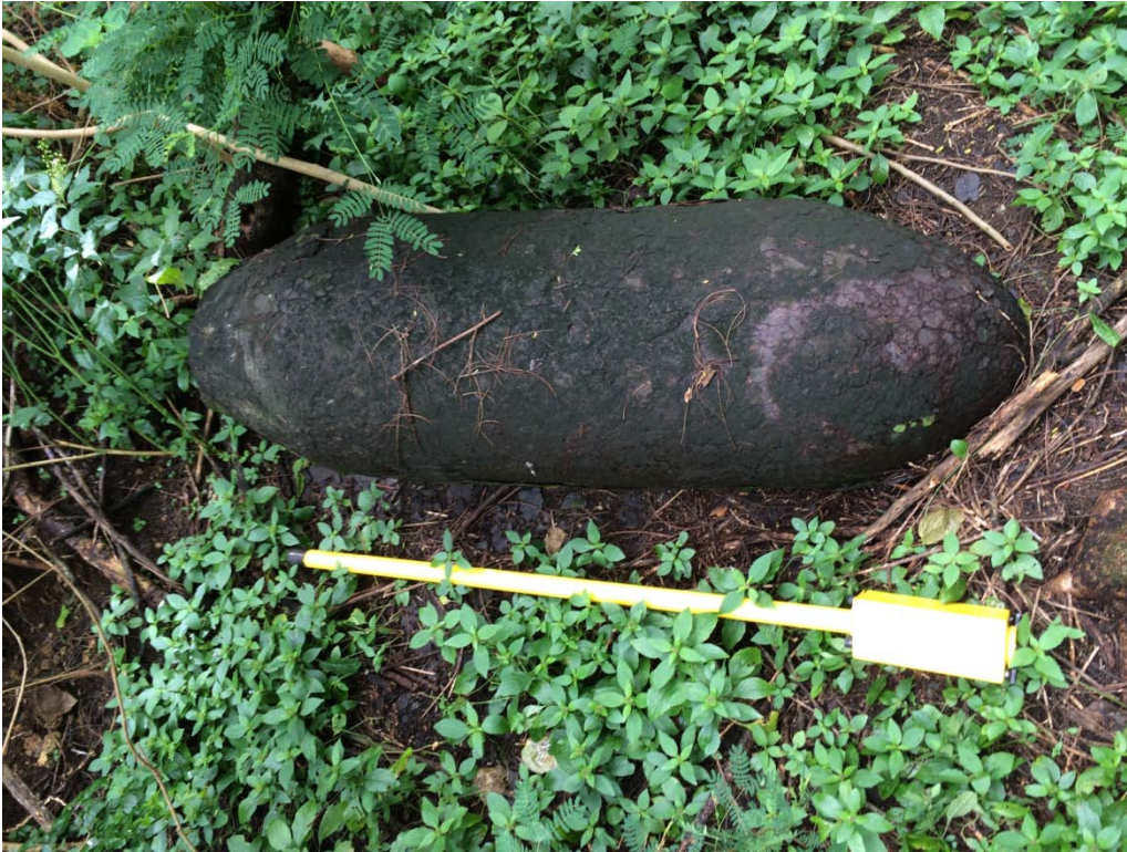
1,000 pound bomb located at soil sample location 093S, with Schonstedts magnetometer shown for scale.
